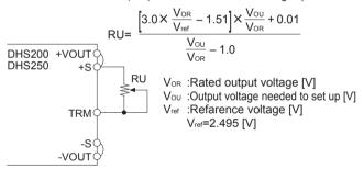
Fig. 3.8 Connection for output voltage increasing (DHS200/250)
