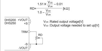
Fig. 3.7 Connection for output voltage decreasing (DHS200/250)
