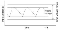
Fig.2.1 Input voltage ripple
