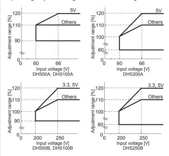
Fig. 3.4 Output Voltage Adjustment Range
