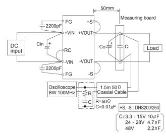
Fig. 2.5 Method of Measuring Output Ripple and Ripple Noise
