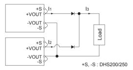
Fig. 4.2 Example of Redundancy Operation
