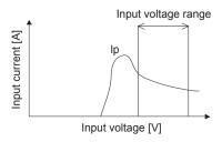
Fig.2.2 Input current characteristics
